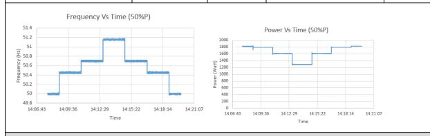
**Power output with falling frequency test:** This test should be carried out in accordance with EN 50438 Annex D.3.2 active power feed-in at under-frequency.
